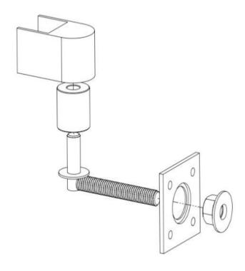
When connecting your large gate using these hinges to your own on-site structure (house, building, column), you will need to purchase your own stainless steel bolts locally based upon the type of material you are mounting it to. Use 3/8" x 5" bolts and locknuts.
